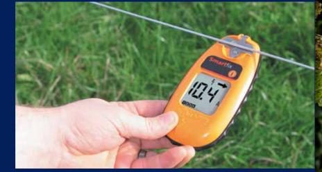
**Use fault finder to monitor voltage and find shorts.** For electric fencing to work properly, a voltage of approximately 5000 volts should be maintained at all times. Shorts in electric fences can cause reduced voltage and can often be difficult to find. A fault finder shows the direction and severity of the of the short. Purchasing a high-quality fault finder is money well spent!
